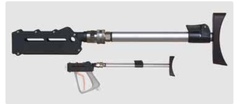
ST-3900 shoulder supports. New European Union guidelines imperatively prescribe the use of shoulder supports for cleaning applications exceeding an operating reaction force of 150 N. Variably adjustable ST-3900. Swiveling coupling. Suitable for guns ST-3600 / ST-3500.
