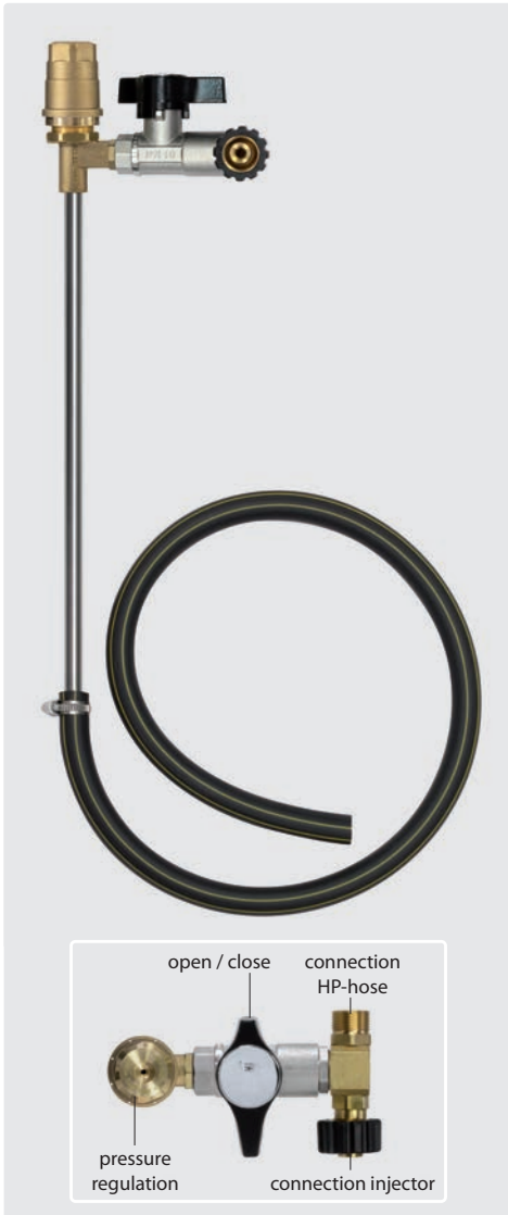
ST-230 with connection, ball valve, stainless steel lance 400 mm and hose 1,000 mm. Max. 250 bar / 30 l/min / 95 °C
