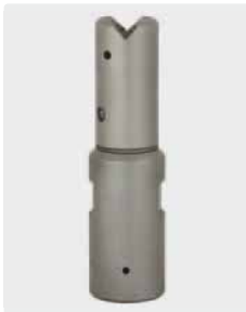
1/8" F. Side jet 2. Front jet 2. Stainless steel. Rotating body hp-bronze. Compact model, universally applicable. Extreme cleaning performance, removes hard deposits. \uparrow 80 mm. \varnothing 12 mm. Weight 0.18 kg. Max. 1000 bar
