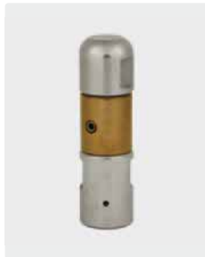
1/8" F. Side jet 2. Stainless steel. Rotating body hp-bronze. Compact model, universally applicable. Extreme cleaning performance, removes hard deposits. \uparrow 63 mm. \varnothing 12 mm. Weight 0.18 kg. Max. 1000 bar
