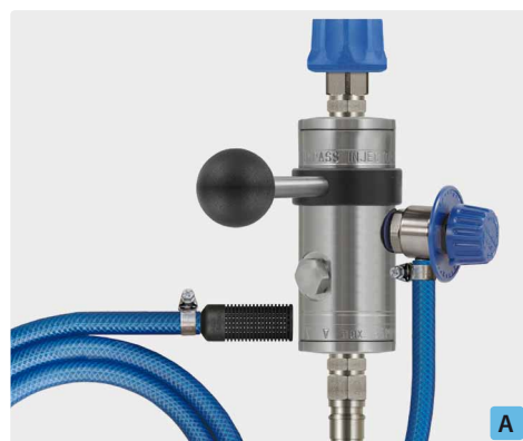
Coupling ST-45-250 nickel-plated brass : plug ST-45-250 stainless steel. Injector ST-167 with metering valve ST-161, suction hose 2,000 mm and suction filter ST-31. Max. 250 bar / 100 °C
