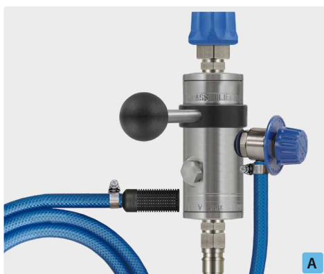
Coupling ST-45-250 stainless steel : plug ST-45-250 stainless steel. Injector ST-167 with metering valve ST-161, suction hose 2,000 mm and suction filter ST-31. Max. 250 bar / 100 °C
