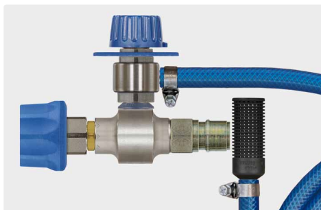
Coupling ST-45-250 nickel-plated brass : plug ST-45-250 zinc-plated steel. Injector with metering valve ST-161, suction hose 2,000 mm and suction filter ST-31. Max. 250 bar / 90 °C
