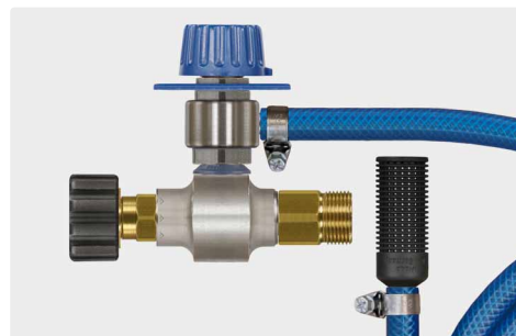
M22 F : M22 M. Injector with metering valve ST-161, suction hose 2,000 mm and suction filter ST-31. Max. 350 bar / 90 °C
