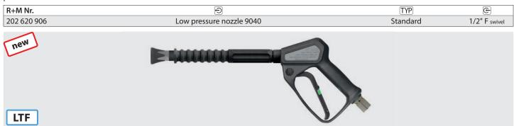
Professional low pressure foam lance with patented LTF technology. Gun ST-2620 with 300 mm insulated lance and nozzle protection ST-10 with lowpressure nozzle 9040. Max. 125 bar / 80 l / min / 150 ° C
