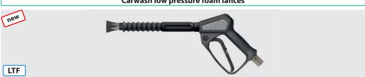
Professional low pressure foam lance with patented LTF technology. Gun ST-2620 with 300 mm insulated lance and nozzle protection ST-10 with lowpressure nozzle 9040. Max. 125 bar / 80 l / min / 150  $^{\circ}$  C
