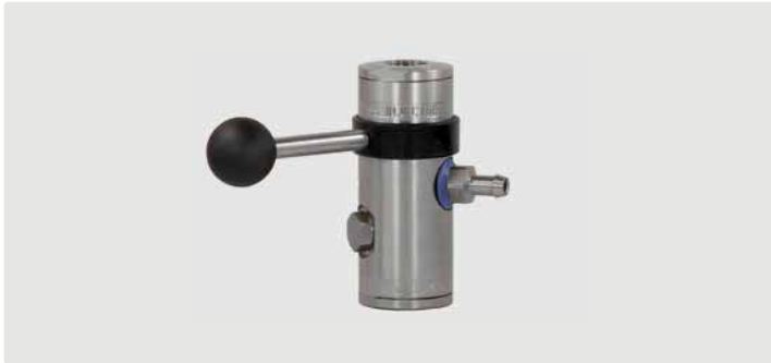
1/2" F : 1/2" F : hose tail 9 mm. The chemical dosing is adjusted by 10 exchangeable nozzle inserts (0.5 - 2.0 mm). Max. 350 bar / 100 °C
