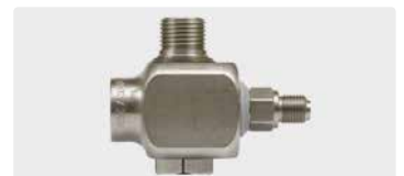
1/4" M : 1/2" M swivel : 1/2" F. Stainless steel. For injection of compressed air. Max. 350 bar / 60 °C
