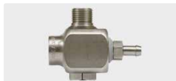
Hose tail 9 mm : 1/2" M swivel : 1/2" F. Stainless steel. For injection of compressed air. Max. 350 bar / 60 °C
