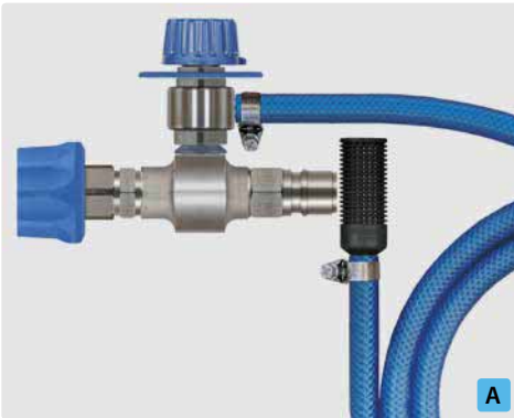
Coupling ST-45-250 nickel-plated brass : plug ST-45-250 stainless steel. Injector ST-160 with metering valve ST-161, suction hose 2,000 mm and suction filter ST-31. Max. 250 bar / 90 °C
