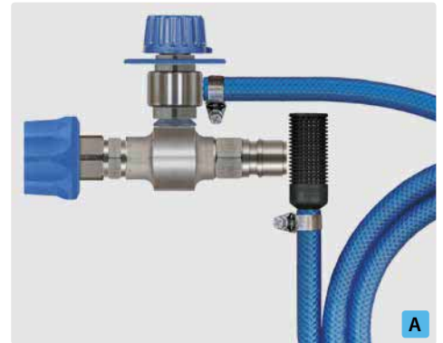
Coupling ST-45-250 nickel-plated brass : plug ST-45-250 stainless steel. Injector ST-160 with metering valve ST-161, suction hose 2,000 mm and suction filter ST-31. Max. 250 bar / 90 °C
