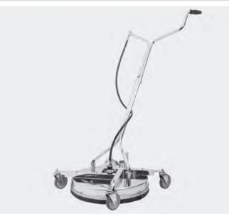
Completely stainless steel. Surface cleaner with an additional frame for highest stability. A height adjustable housing including a device for extraction. Foldable handle bar for space saving and reasonable transport. 2 nozzles are required. Suitable for 50 mm suction hose. 4 industrial castors (100 mm). Max. 2,400 l/h / 120 °C
