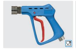
Professional high-flow gun. Gun with coupling ST-45. Stainless steel. Field of application: foam and rinsing applications in the food industry etc. Max. 150 bar / 100 l/min / 150 °C
