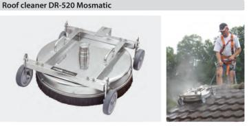
Completely stainless steel. Roof cleaner with an additional frame for highest stability. Adjustable in width of up to 90 mm and in height of up to 33 mm. Including a safety loop for the safety rope with clippers. The use of the ST-550 foot valve is recommended. 4 industrial castors (125 mm). Max. 2,400 l/h / 120 °C
