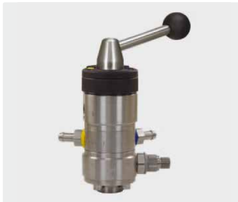
3/8" F : 1/2" F : 2 x Hose tail 9 mm : compressed air module (1/4" M). The chemical dosing is adjusted by 2 x 8 exchangeable nozzle inserts (0.5 - 2 mm). Max. 350 bar / 100 °C
