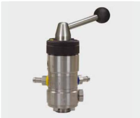
3/8" F : 1/2" F : 2 x hose tail 9 mm. The chemical dosing is adjusted by 2 x 8 exchangeable nozzle inserts (0.5 - 1.5 mm). Max. 350 bar / 100 °C
