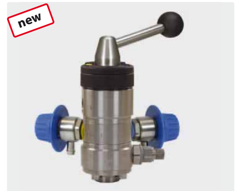
3/8" F : 1/2" F : 2 x Hose tail 9 mm : compressed air module (1/4" M). The chemical dosing is adjusted by the metering valve ST-161. Max. 350 bar / 100 °C
