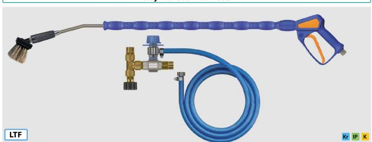
easywash365+ foam set: easywash365+ spray gun, lance and brush with turbofoam365+ air injector by Suttner and injector ST-160 (M22 F and 2 x M22 M) with metering valve ST-161, suction hose 1,000 mm and suction filter ST-32. Max. 310 bar / 90 °C
