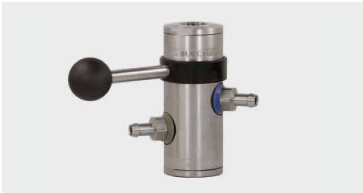
1/2" F : 1/2" F. Injector ST-168 with hose tail 9 mm and compressed air module (hose tail 9 mm). The chemical dosing is adjusted by 8 exchangeable nozzle inserts (0.5 - 1.5 mm). Max. 350 bar / 100 °C
