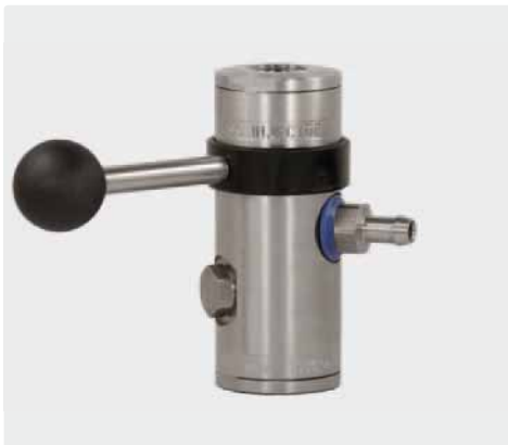
1/2" F : 1/2" F : hose tail 9 mm. The chemical dosing is adjusted by 8 exchangeable nozzle inserts (0.5 - 1.5 mm). Max. 350 bar / 100 °C
