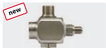
1/4" M : 1/2" M swivel : 1/2" F. Stainless steel. For injection of compressed air. Max. 350 bar / 60 °C
