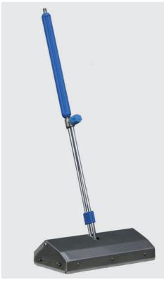
Stainless steel. Variable pressure regulation. Low pressure phase for chemical suction. 4 nozzles 80° 015 included. Width 400 mm. Max. 250 bar / 21 l/min / 80 °C
