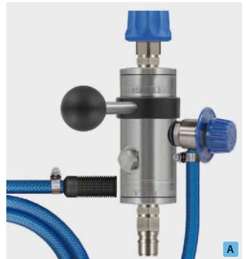
Coupling ST-45-250 nickel-plated brass : plug ST-45-250 stainless steel. Injector ST-167 with metering valve ST-161, suction hose 2000 mm and suction filter ST-31. Max. 250 bar / 100 °C
