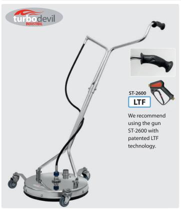
Surface cleaner with foldable handle bar for space saving and reasonable transport. Very robust swivel with triple bearing system and tungsten carbide sealing elements. 3 stainless steel industrial castors (60 mm). 2 nozzles 1/4" M are required.
