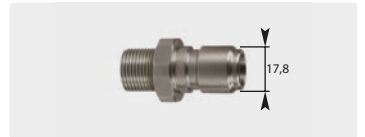
Plug : M. Stainless steel. 60° cone. Max. 250 bar / 150 °C
