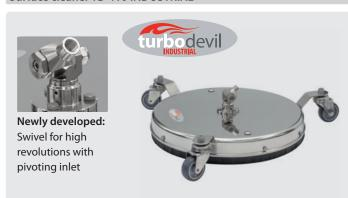
Surface cleaner with a newly developed swivel with pivoting inlet for high revolutions per minute. The bending of the swivel is variably adjustable thus making an easy cleaning of floors and walls possible. 3 industrial castors (60 mm). 2 nozzles 1/4" M are required. Max. 1,800 l/h / 120 °C
