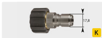
Plug : F. Stainless steel + brass. Max. 250 bar / 150 °C
