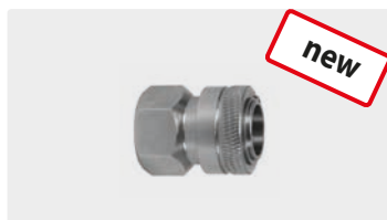
Coupling : F. Stainless steel. Max. 150 bar / 90 °C
