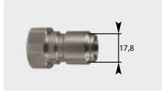
Plug : 1/2" F. Stainless steel. Max. 250 bar / 150 °C
