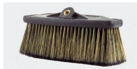
A= 270. B= 260 x 80 mm. Hog hair / synthetic. Max. 40 l/min / 60 °C
