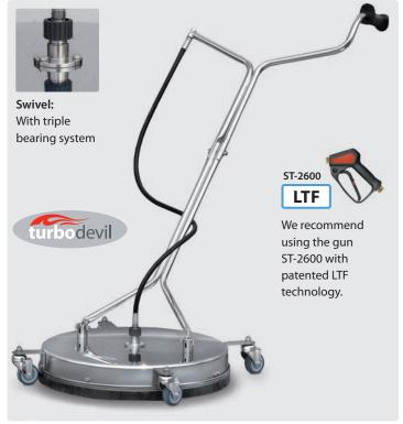
Surface cleaner with foldable handle bar for space saving and reasonable transport. Swivel with triple bearing system. 4 industrial castors (60 mm). 2 nozzles 1/4" M are required.
