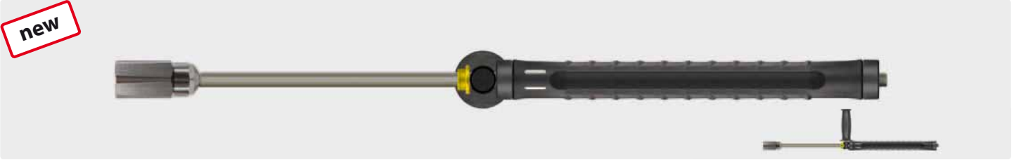
1/4" M. Foam lance stainless steel with air injector, vented handle ST-9.9 330 mm, grip and stainless steel socket with nozzle. A foam injector is required. Max. 250 bar / 80 °C
