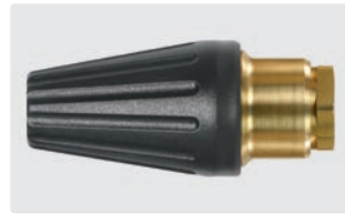
1/2" F. Spray angle 20°. 120 - 250 bar. Max. 100 °C
