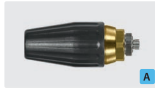
1/8" M. Spray angle 20°. 100 - 250 bar. Max. 100 °C
