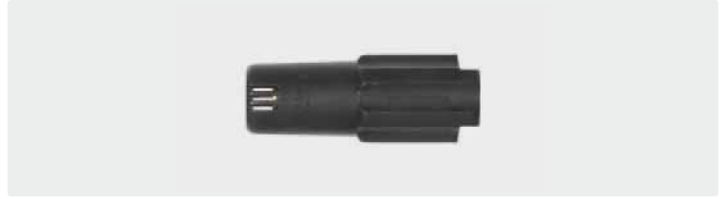
1/4" F. Housing black. Nozzle and seal kit ceramic. Adjustable spray angle. 100 - 250 bar. Max. 80 °C
