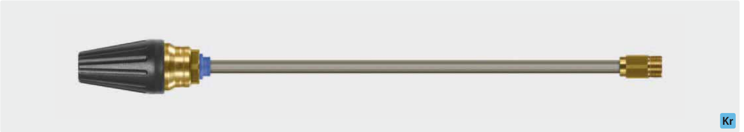
M22 M. Lance with rotating nozzle ST-458.1. Spray angle 20°. 200 - 400 bar. Max. 100 °C
