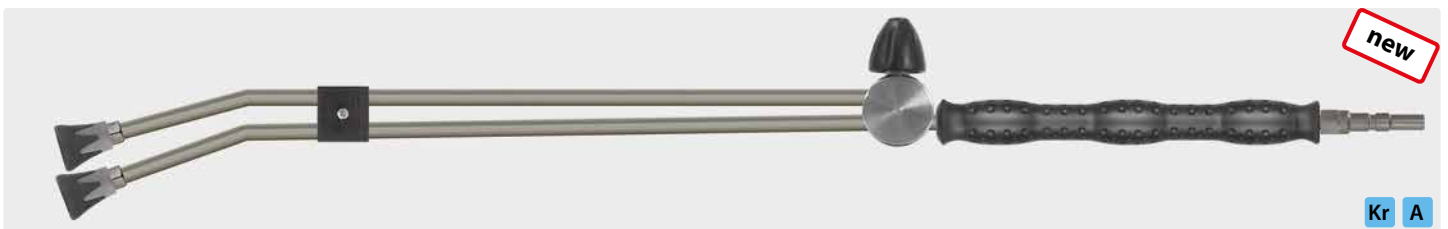
Plug KW. Lance with moulded handle ST-28 Cool & Compact, valve ST-53.2 on top and nozzle protector ST-10 with low pressure nozzle & thread 1/4" F. Max. 400 bar / 150 °C
