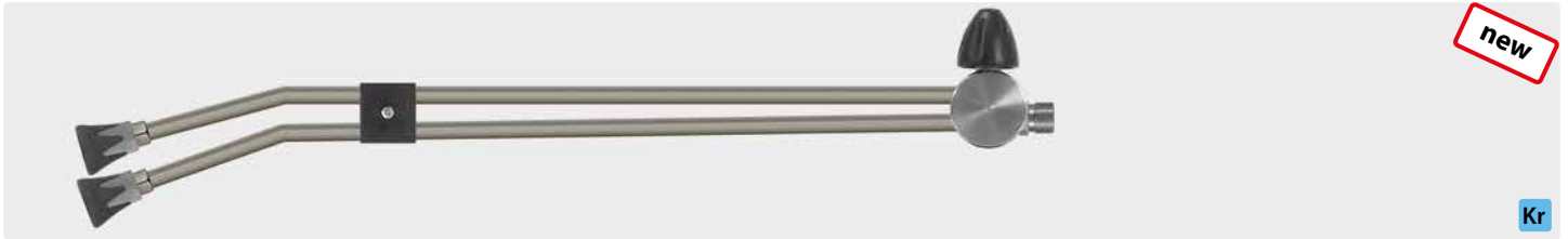
M22 M. Lance with valve ST-53.2 on top and nozzle protector ST-10 with low pressure nozzle. Max.400 bar / 150 °C
