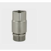
Chrome-plated brass. Backflow preventer according to DIN 19884 and DIN EN 1717. Avoids that cleaning agents come into the potable drink circuit in case of excess pressure in the water pipe. Required when direct connection to pump
