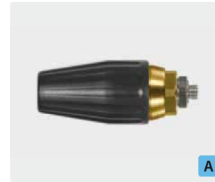
1/8" M. Spray angle 20°. 100 - 250 bar. Max. 100 °C
