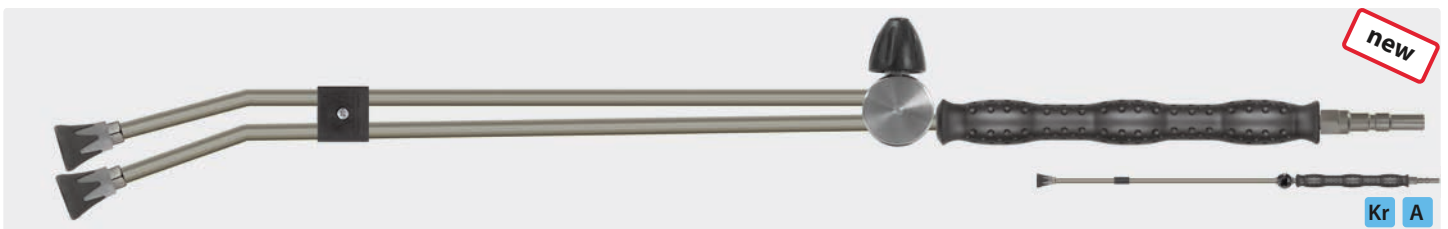
Plug KW. Lance with moulded handle ST-29 Cool & Compact, valve ST-53.2 on top and nozzle protector ST-10 with low pressure nozzle & thread 1/4" F. Max. 400 bar / 150 °C
