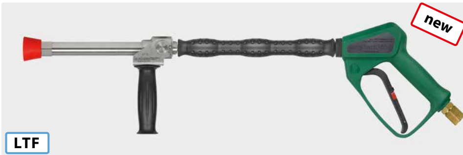
1/2" F. Stainless steel. Longcast lance 300 mm with vented handle ST-29 Cool & Compact 330 mm, gun easyfarm365+, grip aside and nozzle protector made out of plastic without nozzle. Max. 250 bar / 60 l/min / 100 °C
