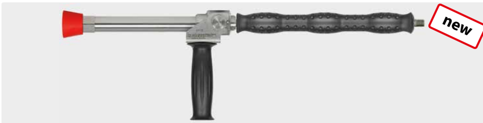
1/4" M. Stainless steel. Longcast lance 300 mm with vented handle ST-29 Cool & Compact 330 mm, grip aside and nozzle protector made out of plastic without nozzle. Max. 280 bar / 130 l/min / 100 °C
