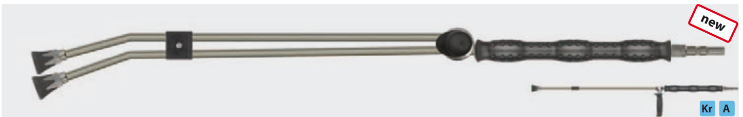
Plug KW. Lance with moulded handle ST-28 Cool & Compact, valve ST-54.2 aside and nozzle protector ST-10 with low pressure nozzle & thread 1/4" F. Max. 400 bar / 150 °C
