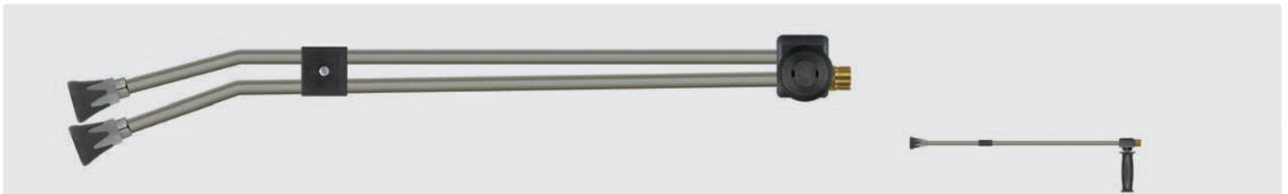
M22 M. Lance with valve ST-54 aside and nozzle protector ST-10 with low pressure nozzle & thread 1/4" F. Max. 310 bar / 150 °C
