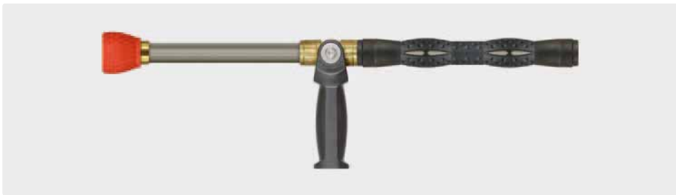
1/4" M. Longcast lance 500 mm with vented handle ST-9.1 260 mm, grip aside and nozzle protector made out of plastic without nozzle. Max. 180 bar / 130 l/min
