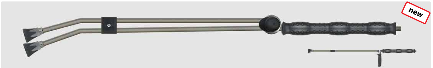
1/4" M. Lance with moulded handle ST-28 Cool & Compact, valve ST-54.2 aside and nozzle protector ST-10 with low pressure nozzle & thread 1/4" F. Max. 400 bar / 150 °C
