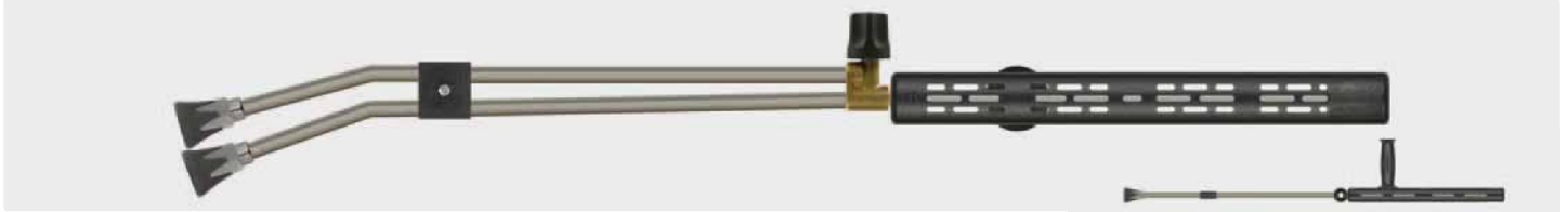
1/4" M. Lance with insulation ST-9 & grip, valve ST-53 on top and nozzle protector ST-10 with low pressure nozzle & thread 1/4" F. Max. 250 bar / 150 °C
