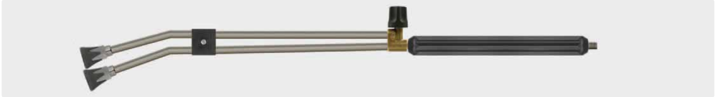
1/4" M. Lance with moulded handle, valve ST-53 on top and nozzle protector ST-10 with low pressure nozzle & thread 1/4" F. Max. 250 bar / 150 °C
