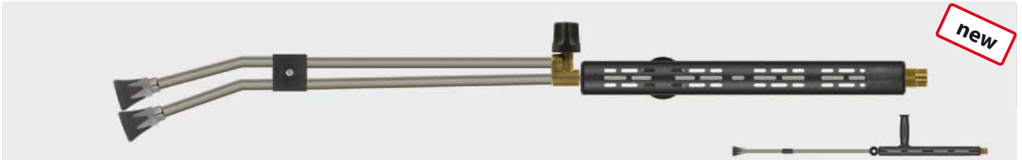
M22 M. Lance with insulation ST-9 & grip, valve ST-53 on top and nozzle protector ST-10 with low pressure nozzle & thread 1/4" F. Max. 250 bar / 150 °C
