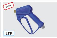
Professional gun. Freeze stop version. With integrated ball bearing swivel. Max. 310 bar / 45 l/min / 150 °C
