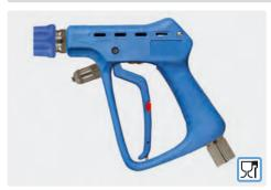
Professional gun with progressive closing system. Gun with coupling ST-3100. Stainless steel. Field of application: foam and rinsing applications in the food industry etc. Industry standard. Max. 60 bar / 100 l/min / 150 °C
