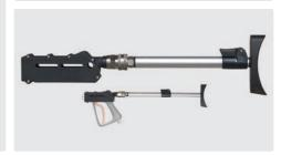
**ST-3900 shoulder supports**. New European Union guidelines imperatively prescribe the use of shoulder supports for cleaning applications exceeding an operating reaction force of 150 N. Variably adjustable ST-3900. Swiveling coupling. Suitable for guns ST-3600 / ST-3500.
