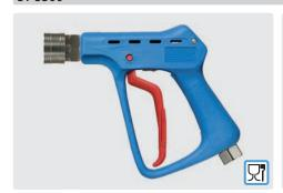
Professional high-flow gun. Gun with coupling ST-45. Stainless steel. Field of application: foam and rinsing applications in the food industry etc. Max. 150 bar / 100 l/min / 150 °C
