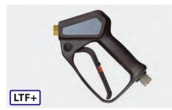
Professional gun. Patented valve kit. Especially wear-resistant ball made out of carbide. Max. 400 bar / 35 l/min / 150 °C
