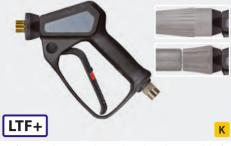
Professional gun with insulated outlet suitable for lances with swivel screw coupling. Patented valve kit. Especially wear-resistant ball made out of carbide. Swivel made out of stainless steel. Max. 400 bar / 35 l/min / 150 °C
