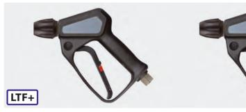
Professional gun with coupling KW. Patented valve kit. Especially wear-resistant ball made out of carbide. Max. 400 bar / 35 l/min / 150 °C
