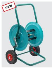
Epoxy powder coated drum and frame. Brass quick couplings. Suitable for 80 meters of hose with a diameter of 3/4" (DN 19) or 60 meters of hose with a diameter of 1" (DN 25) Weight: 11,8 kg
