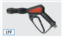
Professional gun with patented LTF technology and Variopress and coupling KW. Variopress regulates the water quantity and serves for the adjustment of pressure. Max. 310 bar / 45 l/min / 150 °C
