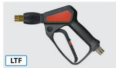
Professional gun with patented LTF technology and Variopress. Variopress regulates the water quantity and serves for the adjustment of pressure. Max. 310 bar / 45 l/min / 150 °C
