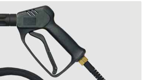
Professional gun with extension 340 mm, max. 210 bar / 25 l/min / 150 °C. Inlet / outlet M22 F. Hose: Flexy (single wire braid), max. 300 bar / 100 °C
