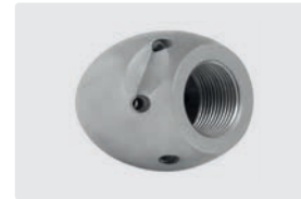
3/4" F. 6x 75° +1x 0°. 30-100 l/min. For \text{R} \text{D} 120-250 mm. Outside \text{D} 50 mm. \text{W} 567 g.
