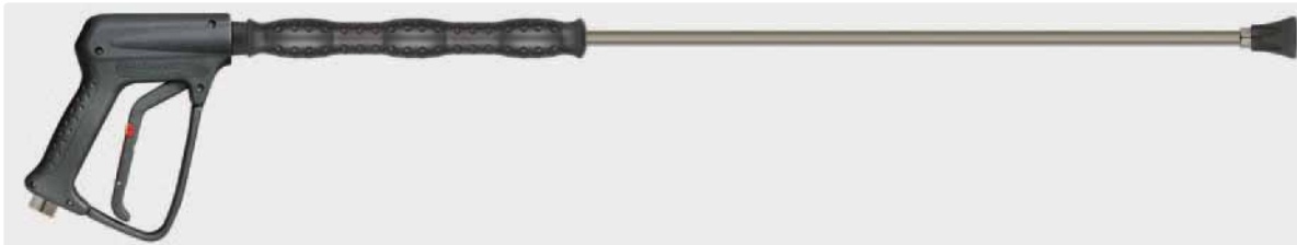
Professional gun R+M EcoLine No. ONE with lance 900 mm zinc-plated steel, insulation ST-28 Cool & Compact 300 mm and nozzle protector ST-10 without nozzle. Max. 250 bar / 45 l/min / 150 °C
