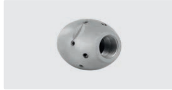
3/8" F. 6x 75° 3x 30° +1x 0°. 30-100 l/min. For \text{R} \text{D} 100-200 mm. Outside \text{D} 35 mm. \text{W} 314 g.
