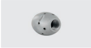
1/4" F. 6x 75° 3x 30° +1x 0°. 25-70 l/min. For \text{R} \text{D} 75-150 mm. Outside \text{D} 30 mm. \text{W} 223 g.
