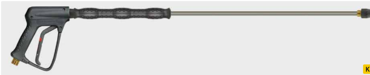
Professional gun R+M EcoLine No. ONE with lance 900 mm zinc-plated steel, insulation ST-28 Cool & Compact 300 mm and nozzle protector without tip. Max. 250 bar / 45 l/min / 150 °C
