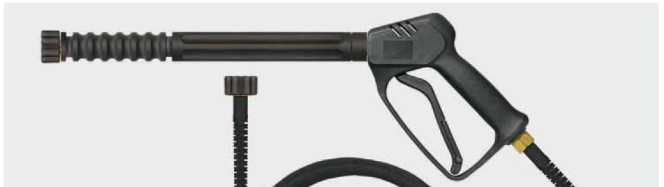
Professional gun with extension 340 mm, max. 210 bar / 25 l/min / 150 °C. Inlet / outlet M22 F. Hose: 6 - 160 (single wire braid), max. 160 bar / 20 °C
