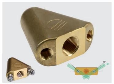
Fitted with two rear facing fan jets the small plough jet nozzle is great for desilting drains and sewers. The heavy forged brass construction keeps the jet firmly planted in the base of the pipe where the silt deposits collect and blasts them back towards the manhole.
