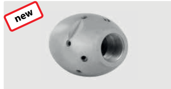
1/2" F. 6x 75° 3x 30° +1x 0°. 80-140 l/min. For \text{R} \text{D} 120-250 mm. Outside \text{D} 40 mm. \text{W} 630 g.
