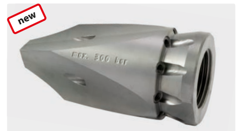
300 bar. 1" F. For tubes > 100 mm Lateral front jets with hardened stainless steel nozzle inserts
