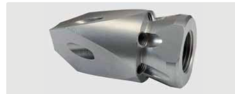
350 bar. 3/8" F. For tubes > 50 mm. Lateral front jets with hardened stainless steel nozzle inserts
