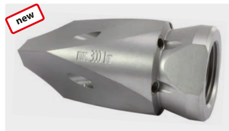
300 bar. 3/4" F. For tubes > 60 mm Lateral front jets with hardened stainless steel nozzle inserts
