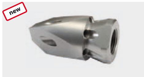
3/8" F. For tubes > 50 mm. Lateral front jets with hardened stainless steel nozzle inserts.
