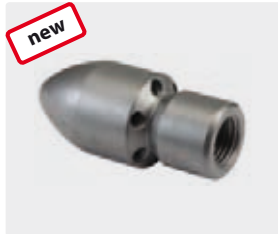
1/4" F. Outside \varnothing 25 mm. 6 rear jets
