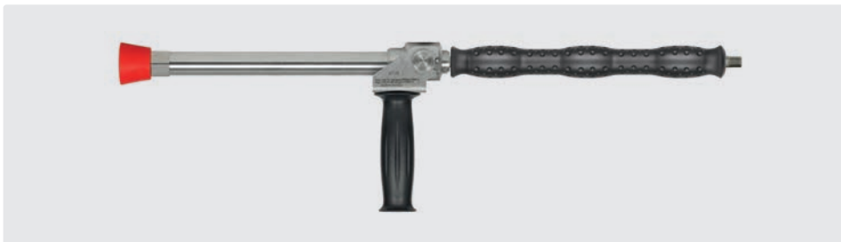
1/4" M. Stainless steel. Longcast lance 350 mm with insulation ST-29 Cool & Compact 330 mm, grip aside and nozzle protector made out of plastic without nozzle. Max. 280 bar / 130 l/min / 100 °C
