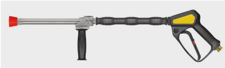
3/8" F. Stainless steel. Longcast lance 350 mm with insulation ST-29 Cool & Compact 330 mm, gun ST-2300, grip aside and nozzle protector made out of plastic without nozzle. Max. 280 bar / 45 l/min / 100 °C
