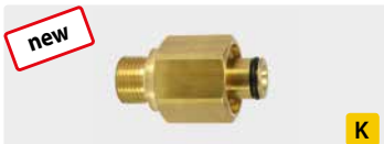
3/8" M : TR22 F. K-Lock 5. Brass. Max. 400 bar / 150° C
