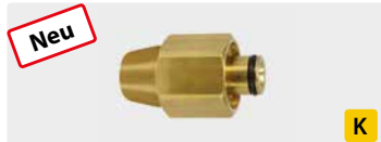
3/8" IG : TR22 IG. K-Lock 5. Messing. Max. 400 bar / 150° C
